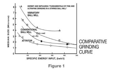
Comparisons of the effectiveness of grinding devises for the ultrafine grinding of Pima chalcopyrite.
